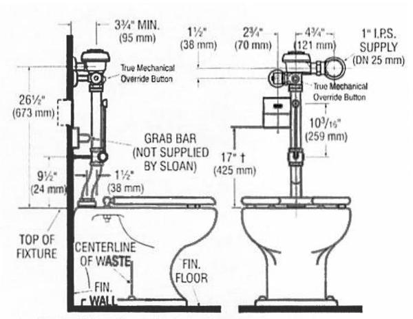
† Position of Sensor Box can be raised or lowered 1" (25 mm) if in conflict with Handicap Grab Bars.
